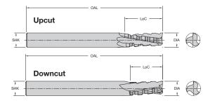
Phenolic materials, an organic resin based material, are used in various industrial applications due to their high strength, corrosion resistance, and insulation properties. Routing this material proves challenging due to its dense nature and high resin makeup, which reduces tool life.
