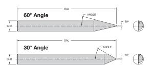
The half round engraving tools are offered with a wide range of tip sizes and angles to accommodate many engraving styles.
